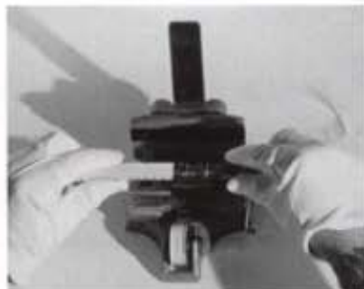
6. Remove filmstrips, now taped together on one side, reverse and re-thread the sprockets on the reverse side. Repeat steps 4 and 5 to make a double-splice, with the strips taped on both sides.
