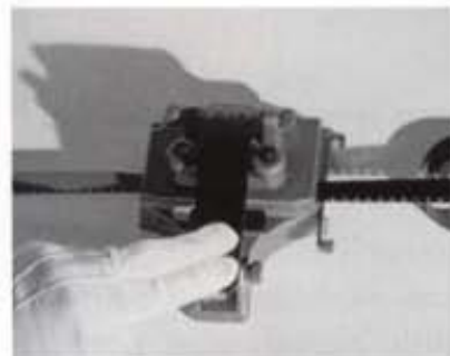
5. Close splicer over taped joint and press lever firmly.
