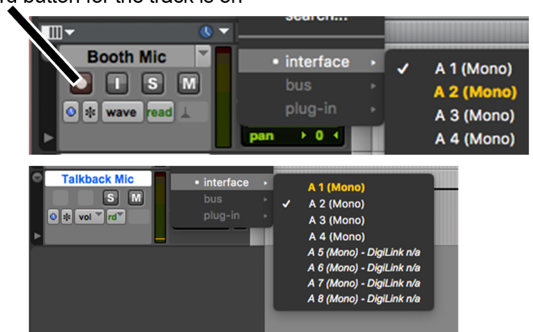
ADR Recording template with Booth Mic on A1 and Talkback Mic on A2
