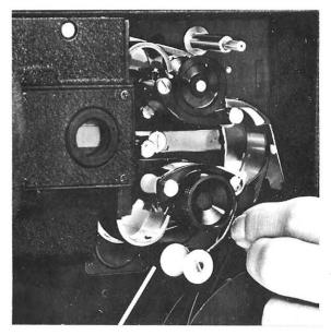
5. Have the filming speed at 16 or 24 fps. Make sure the film holder on the side of the takeoff spool shaft is in the proper position. Push the film slightly while pressing the shutter button.
