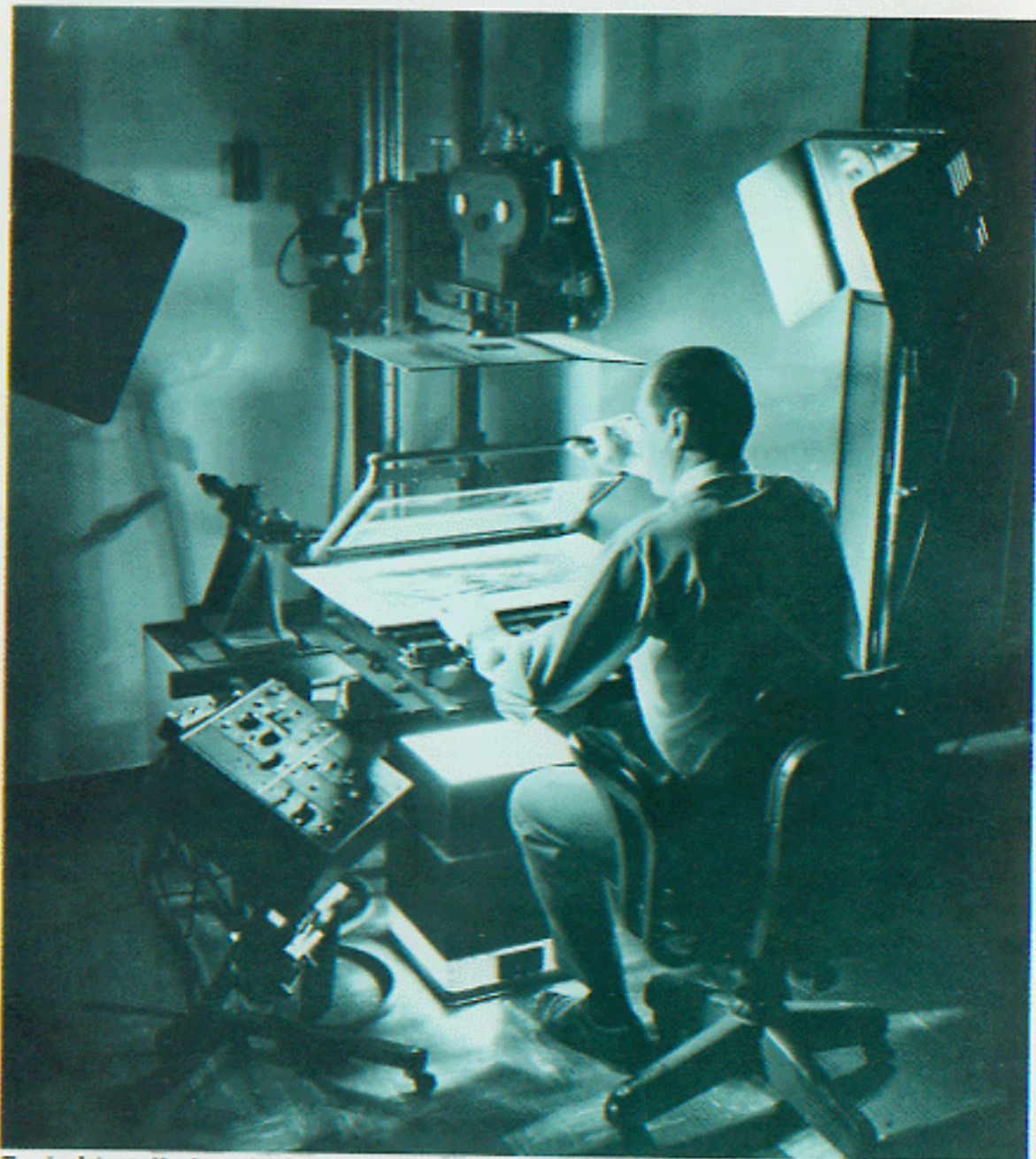
Typical installation of Model 5332-00 16mm Animation Stand and Camera with optional Rollaway Unit and Underlighting Unit. Photo courtesy of AMERICAN AIRLINES audio-visual department.
