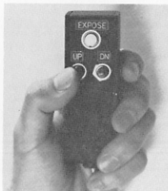
figure 20. Hand Control for camera positioning and film exposure.
