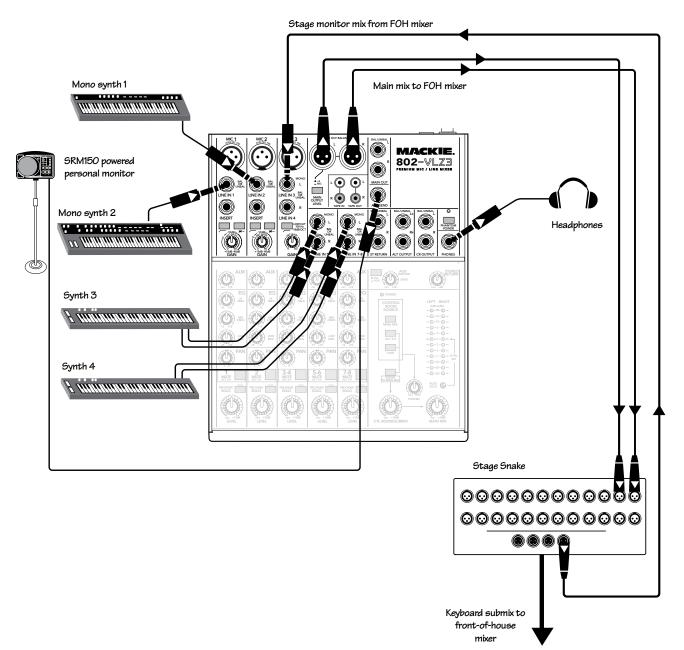
This diagram shows mono synths connected to the mono line inputs of channel 1 and 2, and stereo synths connected to the stereo line inputs of channels 5/6, and 7/8.
