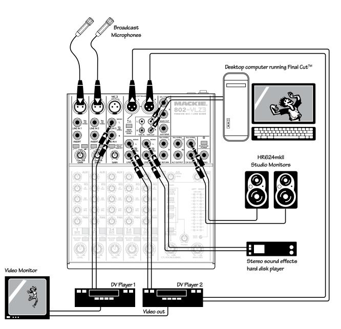
This diagram shows two voice-over microphones connected to the mic inputs of channels 1 and 2. The stereo line-level outputs from two digital video players connect to the line inputs of channels 3/4, and 5/6.
