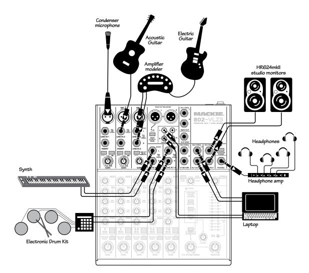
This diagram shows a condenser microphone connected to the mic input of channel 1, with phantom power engaged. A guitar is attached to the instrument input of channel 2, with the instrument switch pressed in. Another guitar plays through an amplifier modeler into channels 3 and 4. A stereo synth is connected to the line inputs of channels 5 and 6, and an electronic drum kit feeds channels 7 and 8.
