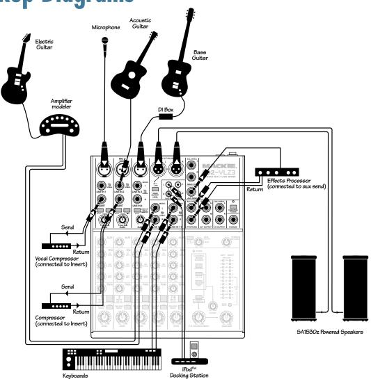
This diagram shows a microphone connected to the mic input of channel 1, and a vocal compressor connected to the insert jack. A guitar is attached to the instrument input of channel 2, with the instrument switch pressed in, and a compressor on the insert. A bass guitar is connected to channel 3's mic input via a DI box, and another guitar plays through an amplifier modeler into channels 5 and 6. Keyboards are connected to the line inputs of channels 7 and 8.
