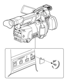
**3** Use the USB cable supplied with the PMW-EX1 to connect the rightmost USB connector to the USB port on the computer.
