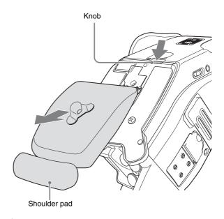
**2** Remove the fixing plate after loosening the screw, then while holding the knob pressed down, pull out the shoulder pad until the notch appears.
