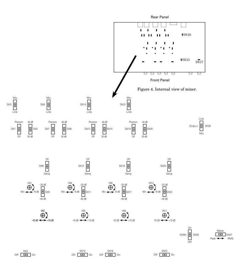
Figure 5. Detail of internal controls.
