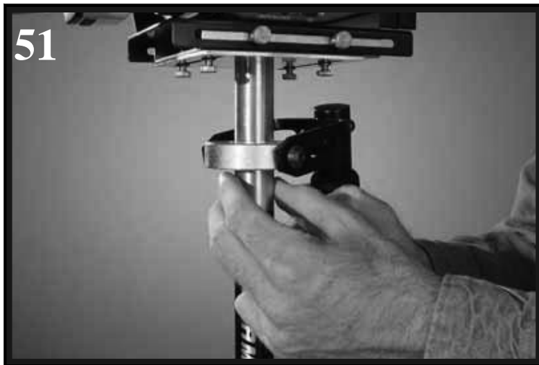
Notice how the “Guiding Hand” does not touch the main bearing assembly or yoke which can be seen just slightly above the fingers of the “Guiding Hand” in Photo # 51.
