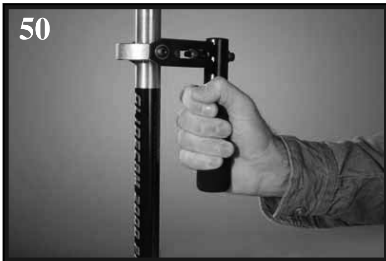
Photo # 50 shows you the correct way to hold the handle, however remember that you should always use both hands when using the 2000 Pro as in Photo # 51.
