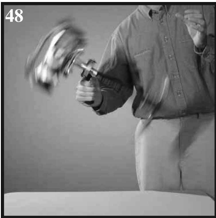
Photo # 48 shows the Glidecam 2000 Pro swinging between horizontal and vertical during the "Sled Arc Test" (see next page).
