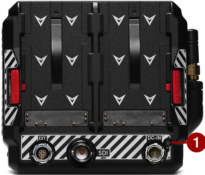
Figure: KOMODO 6K, DC/Battery LED
