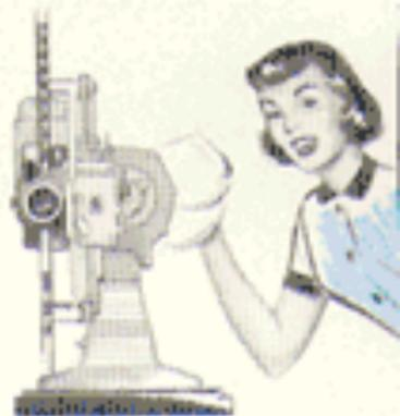
**LENS.** To remove, turn lens lock counter-clockwise (arrow) and pull lens barrel forward gently. To clean, use tissue or cleaning fluid. To replace lens, push it back into position, then tighten lens lock.
